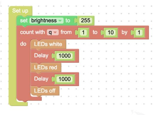
'Set up' is the run block that will only run one time.
