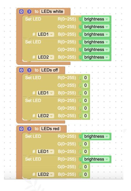
3 functions are defined here, one for each LED setting. Functions are useful and can be called again and again and can work with other functions.
