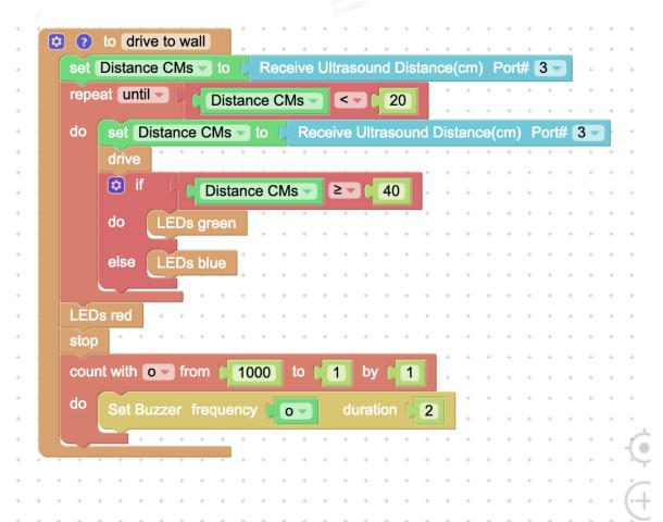
UltraSound Sensors located in the FlipRobots eyes sence the distance(cm) to the object in front of them. We are saving this value in the 'Distance CMs' variable
