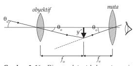
**Gambar. 3. 16.** *Diagram sketsa teleskop astronomis* (*Tipler*, 1991)
