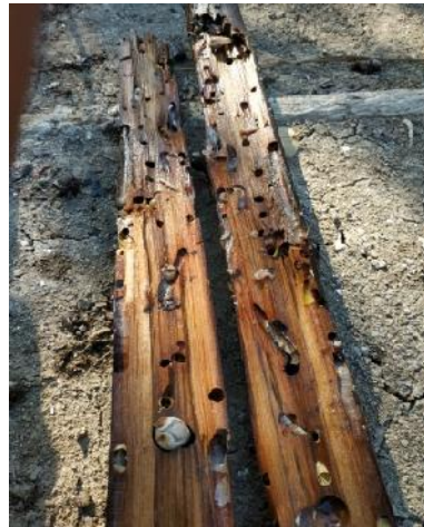
Figure 20. Wood attack by marine wood borer in mangrove forest of Kalimantan Island
